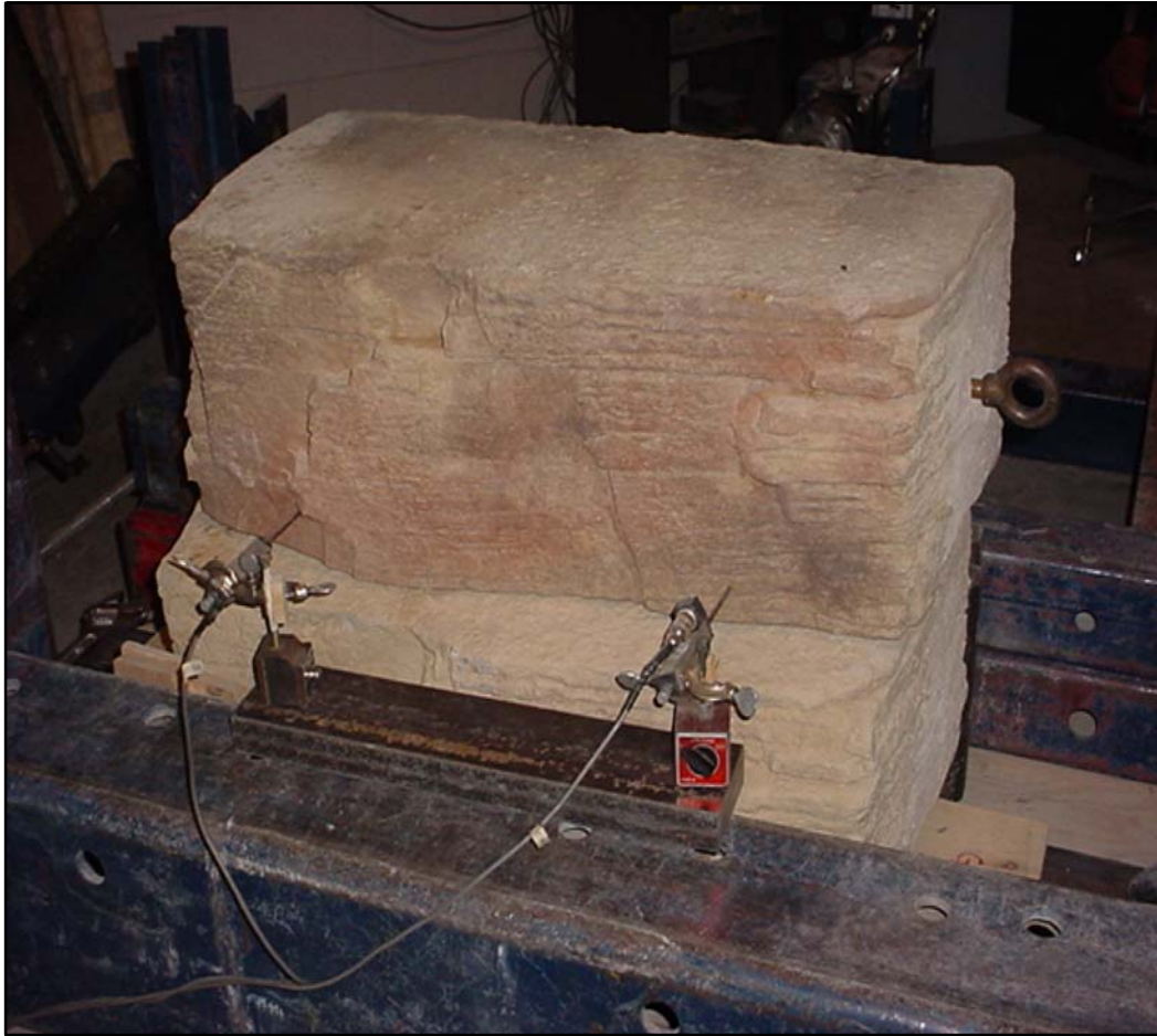
Figure 2: Photograph of the Rosetta block configuration used in the shear test apparatus
